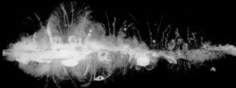
Simulated wound channel in gelatin block / bullet performance in gelatin
